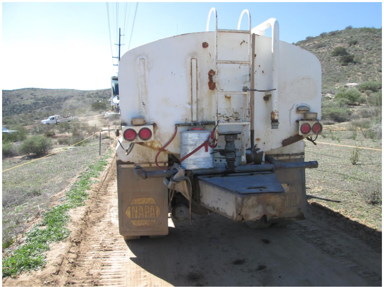
Photo 7: Fire Watch/water tenders were observed adjacent to vegetation trimming activities and construction activity in accordance with the project Fire Plan and APM HAZ-2.
